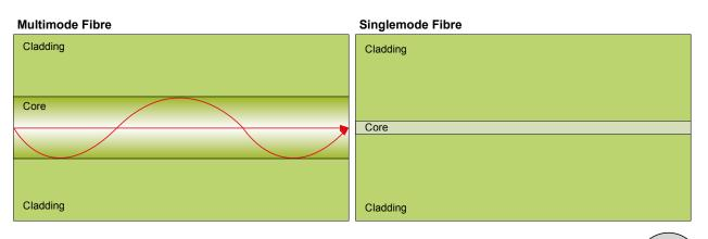
The fibre core comprises of a core and a cladding. This cladding is then covered by a primary coating.
